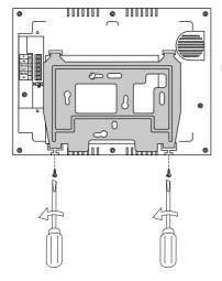
Unscrew the monitor bottom screws.
